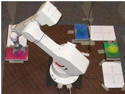
Figure 4. Task Setup: Robot, balls in home positions, and target markers
