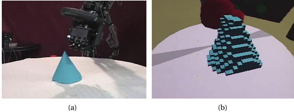
Figure 6-9: Shape reconstruction from multiple views leading to a voxelized shape model
