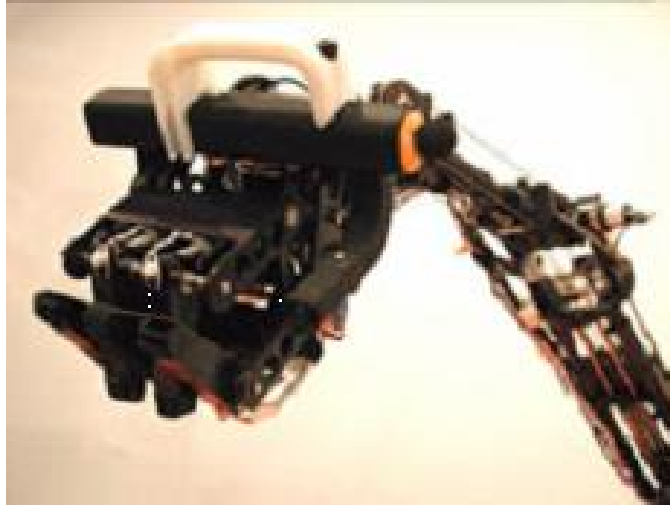
Figure 6-2: Ripley's head - manipulation handle, gripper, cameras mounted at the sides of gripper
