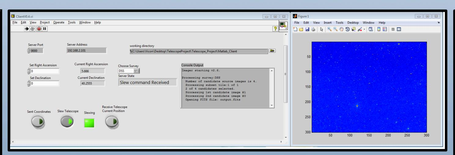
The above image (left) shows a client window representing a telescope control unit of a telescope node of the network. The node has slewed into position and acquired an image (right). The image is then processed to simulate the view of a small aperture telescope, weather conditions, etc. On the far right we see a visualization of the sky of the telescope field of view and pointing using the Stellarium virtual observatory software.
