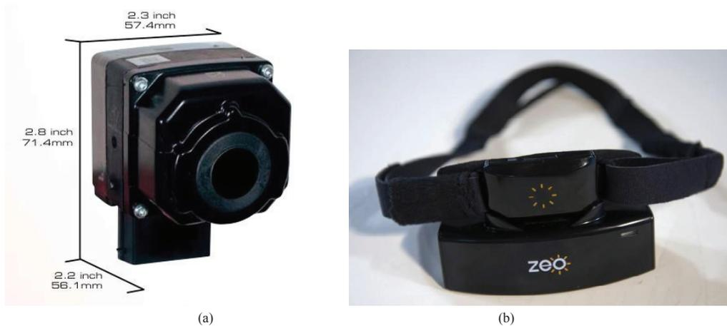
Fig. 2. Experimental equipment. (a) IR thermal imaging camera; (b) EEG device
