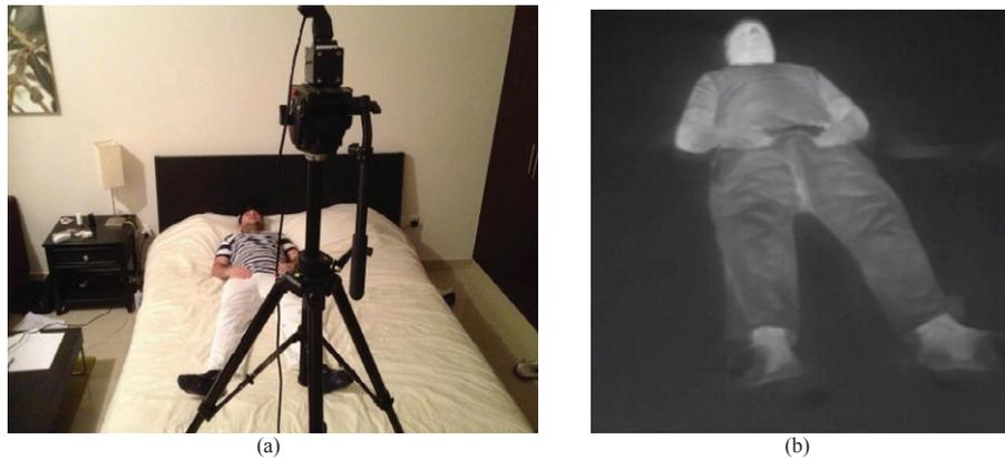
Fig. 3. Experiment environment. (a) experimental setup: FLIR Camera & Strap; (b) infrared image of subject
