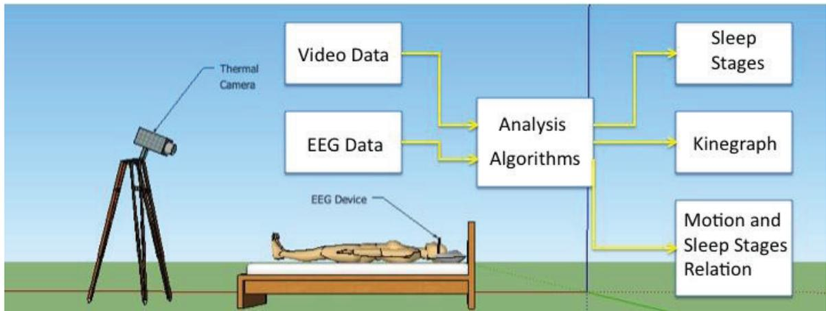
Fig. 1. System Architecture: experimental subject, infrared camera, EEG strap, analysis algorithms, and results
