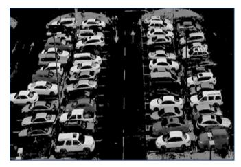
Fig. 3. Pavement pixels subtracted
