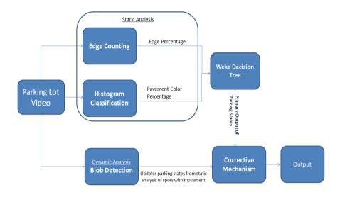
Fig. 6. Block diagram of algorithm mechanism
