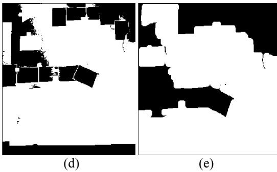
Fig. 4. Algorithm results. a) Initial stitched image. b) Value (third dimension) of the initial map. In this case is the best parameter to use in the segmentation. c) Value equalized. d) Value equalized binarized. e) Same as d) after the closing operation and with the goal point in the (1,1) coordinates of the image.
